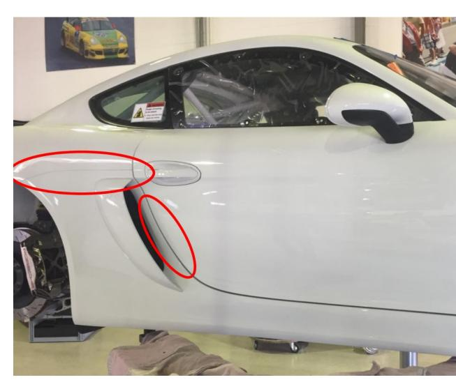
11. Place the appropriate grille into the cavity, slip the grille over the dividing septum. Then replace the panel in the reverse order. Complete!!
