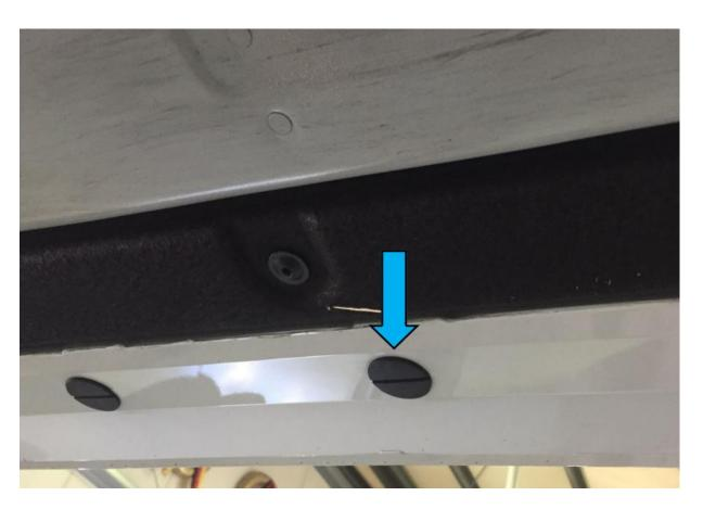
10. On the areas marked red, the door sill is fixed in holding strips by means of snap-in lugs. Carefully pull the door sill out of the retaining tabs.
