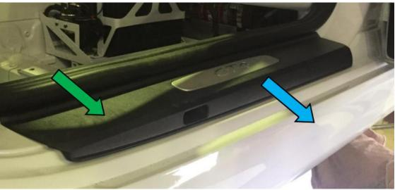
6. Remove the four black plastic spreading rivets with a suitable tool, we recommend a plastic trim removal tool.
