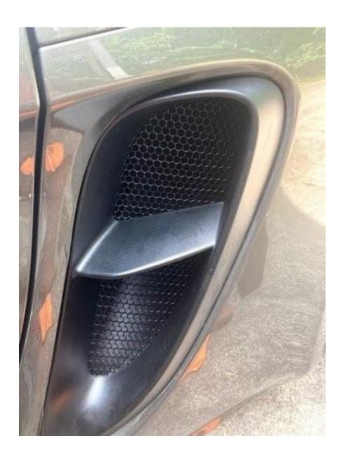
3. The GT4 requires the side sill removal, the piece that houses the trim piece and scoop and runs along the lower rocker of the car. We will highlight the GT4 installation as the GTS and Spyder only require removal of the trim pieces, install the grille, then replace the trim piece.
