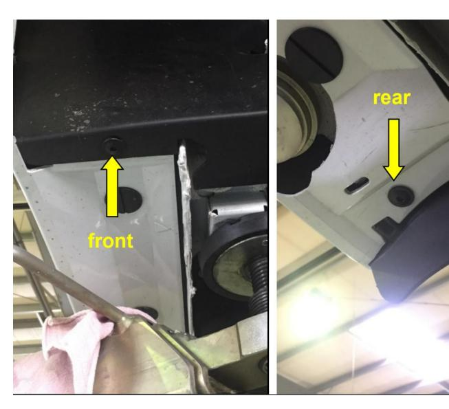
9. Remove all large plastic clips at the bottom of the door sill by twisting them (90°).
