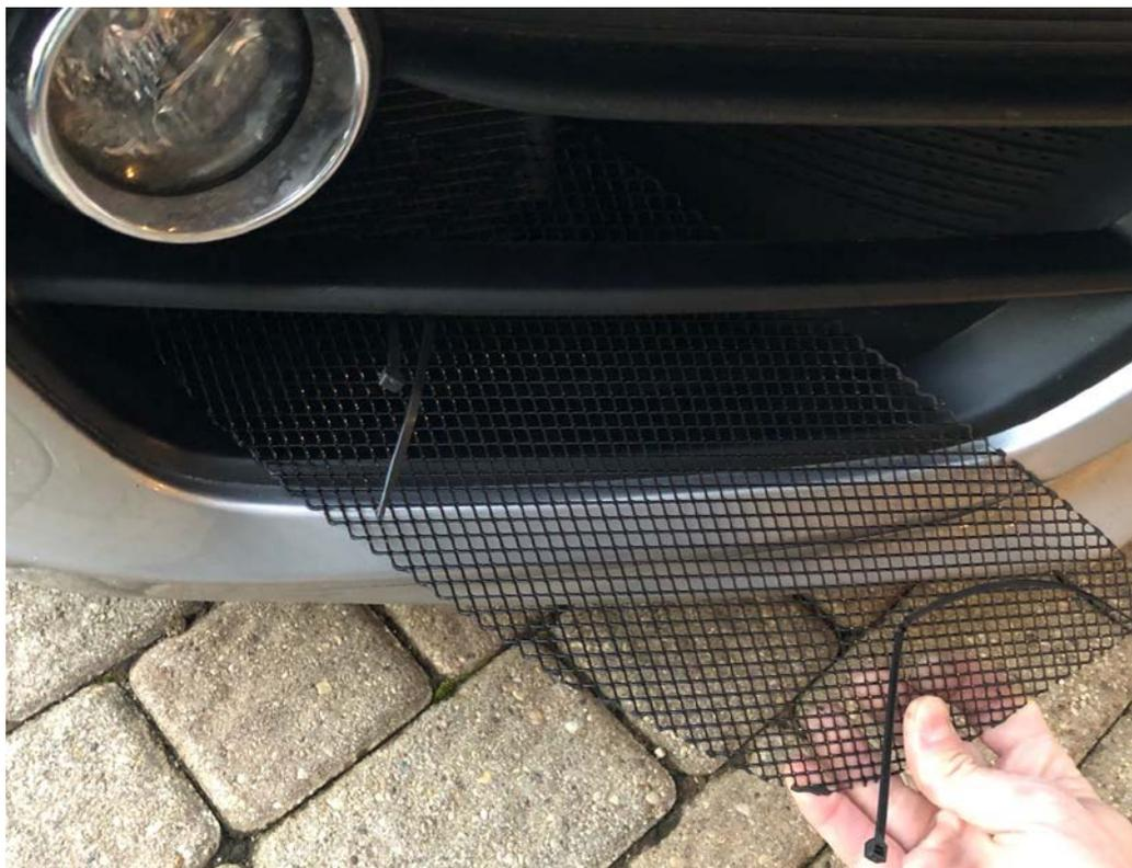
2. Cable ties are preinstalled for ease of installation. Insert hand into space above the middle rib. You will find that using your hand to guide the grill mesh up and to the outside of the car will assist with installation. Do not force the grill. Once the grill is inserted, you will be able to rotate the side in your hand into the cavity of the radiator intake.
