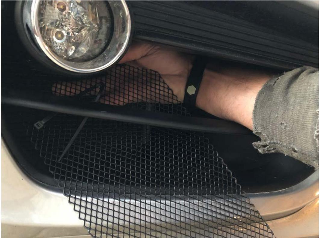
3. The cable ties can be hidden if you would like. The middle bar is two pieces. You can split the bar a part and you will slip the cable ties in between. The receiving end of the cable tie will be on the bottom of the lower bar.
