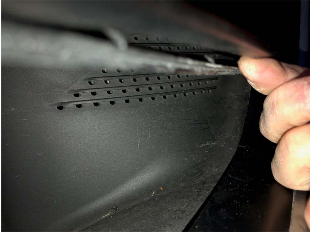
4. Pull the grill towards the front opening and align as you see fit. Insert the cable ties as shown.
