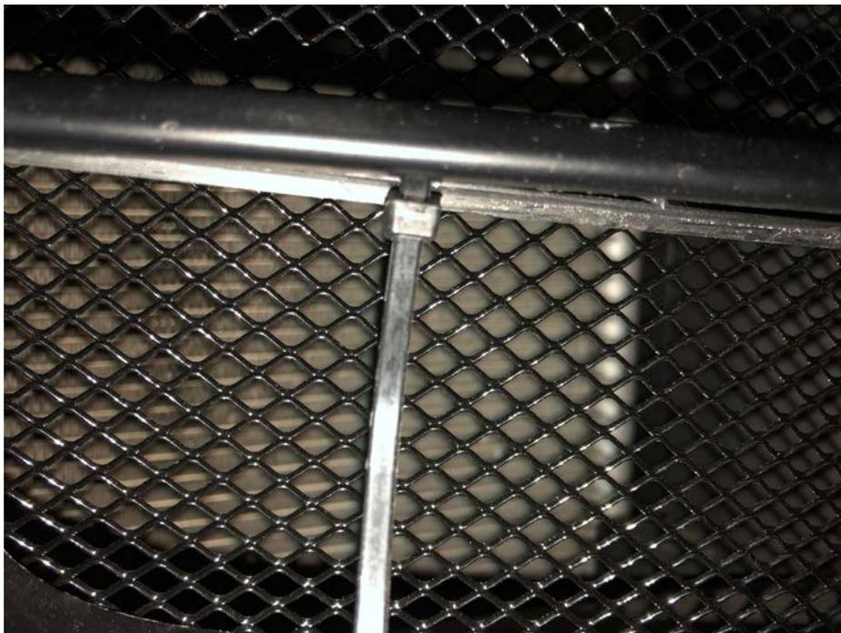
5. Should look like the photo below. Then using a side cutter, clip off the extra cable tie tail.
